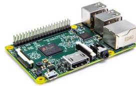
raspbx server (Asterisk + FreePBX on Linux)
